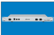
• ID-RP2C REPEATER CONTROLLER Connect to ID-RP2V, ID-RP2V, ID-RP2L and/or Gateway PC.
