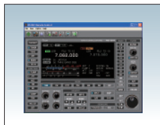
RS-BA1 IP REMOTE CONTROL SOFTWARE For IP remote transceiver control from a PC.
