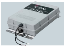
AT-140 HF AUTOMATIC ANTENNA TUNER Covers 1.6–30MHz with a 7m (23 ft) or longer wire antenna. AT-130/E is also available.
