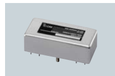
FL-52A CW NARROW FILTER Center freq.: 455 kHz Bandwidth: 500 Hz/–6 dB
