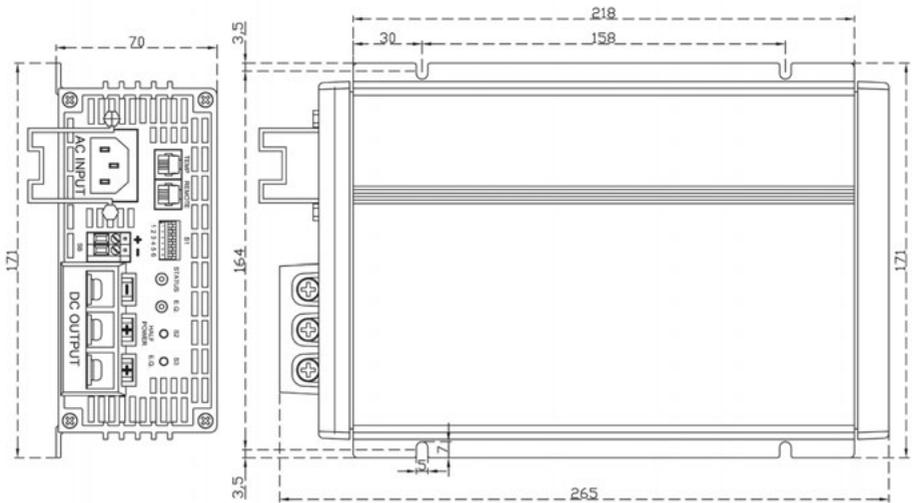
Figure 6 WSC-1230 / WSC-2415 Charger Top View (mm)
