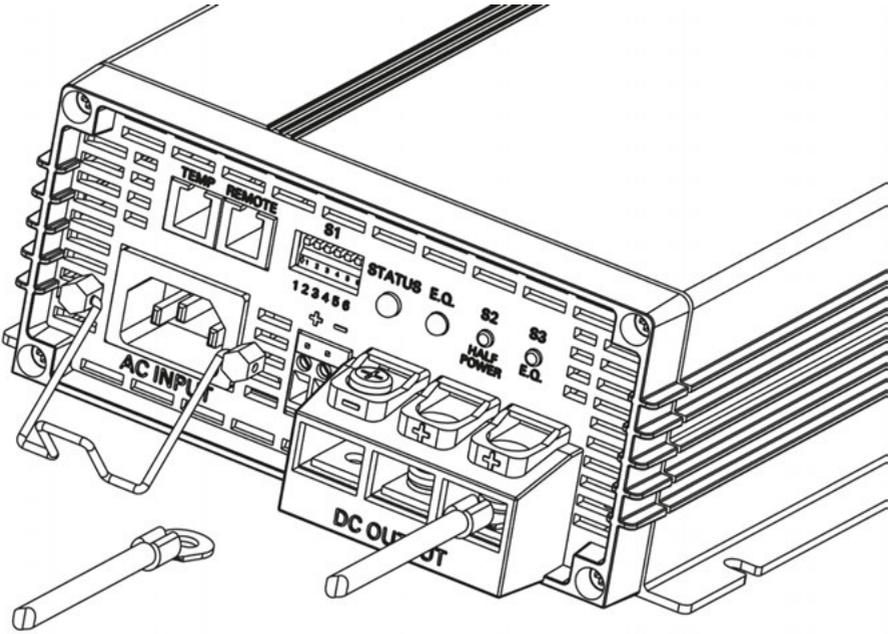
Figure 9 Cable Setup
