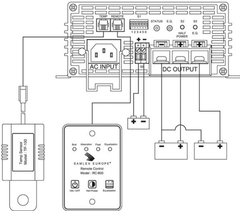
Figure 8 Making Connections
