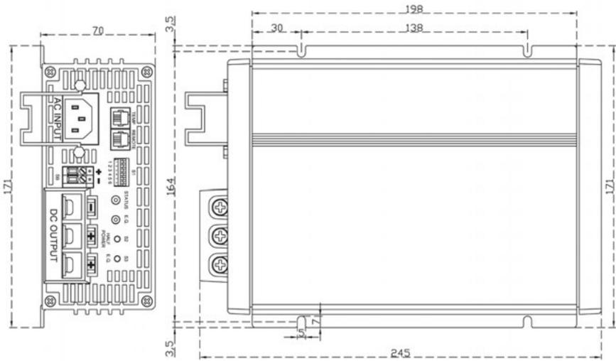
Figure 4 WSC-1215 / WSC-2408 Charger Top View (mm)
