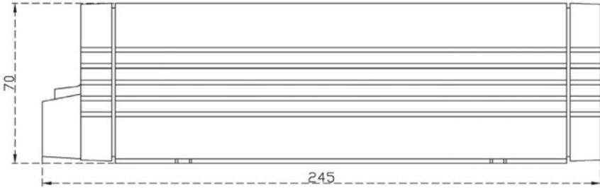
Figure 5 WSC-1215 / WSC-2408 Charger Side View (mm)
