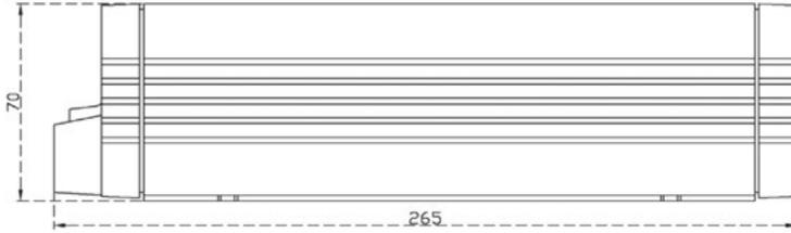
Figure 7 WSC-1230 / WSC-2415 Charger Side View (mm)
