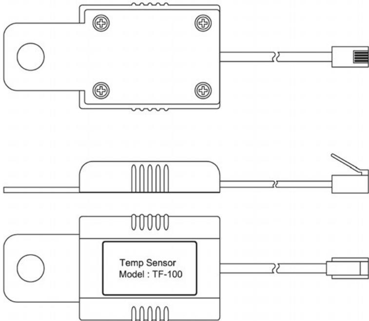
Figure 12 Temperature Sensor TF-100
