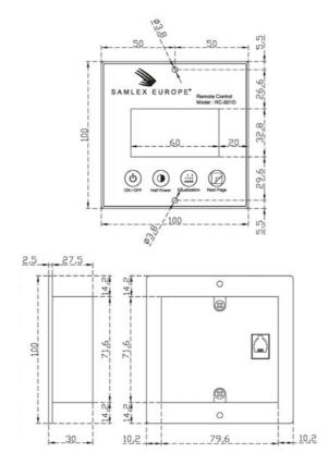
Figure 16 Remote Controller RC-601D Dimension (mm)
