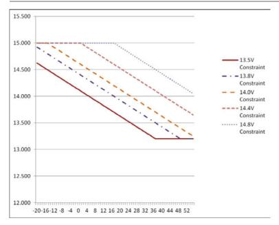
Figure 20 Temperature Compensation for 12V Model
