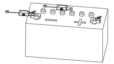
Figure 18 Temperature Sensor Setup
