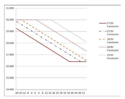
Figure 21 Temperature Compensation for 24V Model
