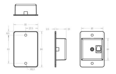
Figure 14 Remote Controller RC-600 Dimension (mm)
