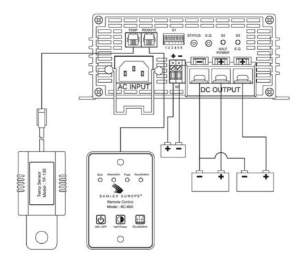
Figure 8 Making Connections
