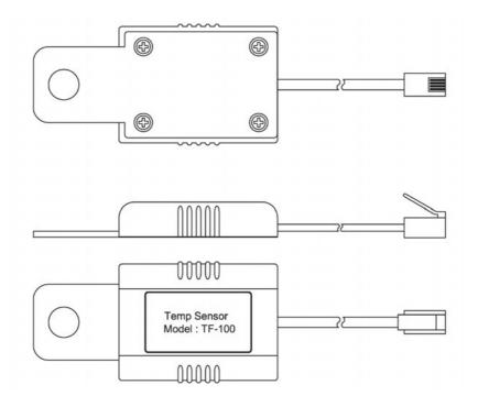
Figure 12 Temperature Sensor TF-100
