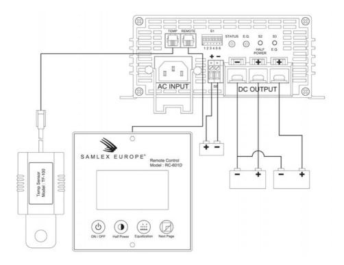
Figure 17 Making Connections (RC-601D)
