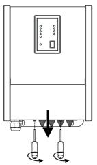
To access the connection compartment, remove the two screws indicated on the left and slide the red connection compartment cover downwards.
