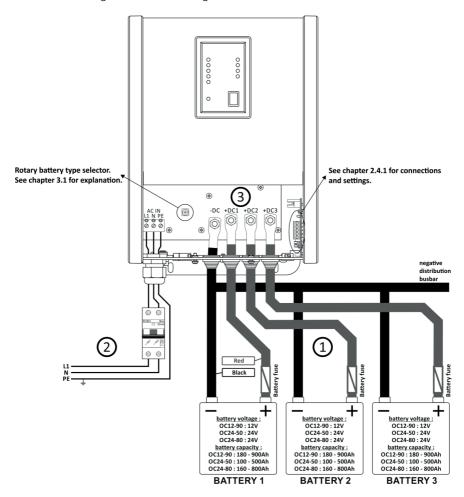
① Please consult the following table to determine the correct battery cable and fuse size for each model. Using a smaller cable size or a longer cable will cause additional losses and may result in improperly charged batteries. Fire and burning hazards are present if the battery cables are insufficiently sized for the expected current. Battery cable lengths longer than 6 meters, are not recommended.
