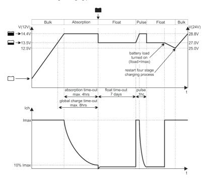
In the Bulk stage, the charger delivers full output current and typically returns approximately 80% of charge back into the battery once the absorption voltage is reached. During this stage, indicators 3d and 3c (see frontpanel image in chapter 4.1) will be lit depending on the Bulk charge progress.
